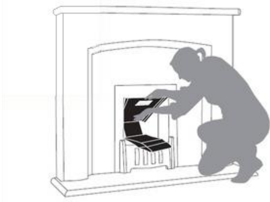
Figure A.4: Chimney Snug
