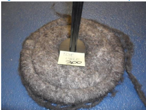
Figure 2.1: Difference between Chimney Sheep at start of BSRIA trial and after 300 cycles
