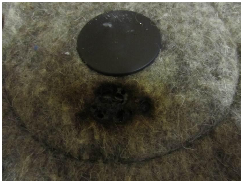
Showing damage on top side of chimney sheep after crib 7 test
