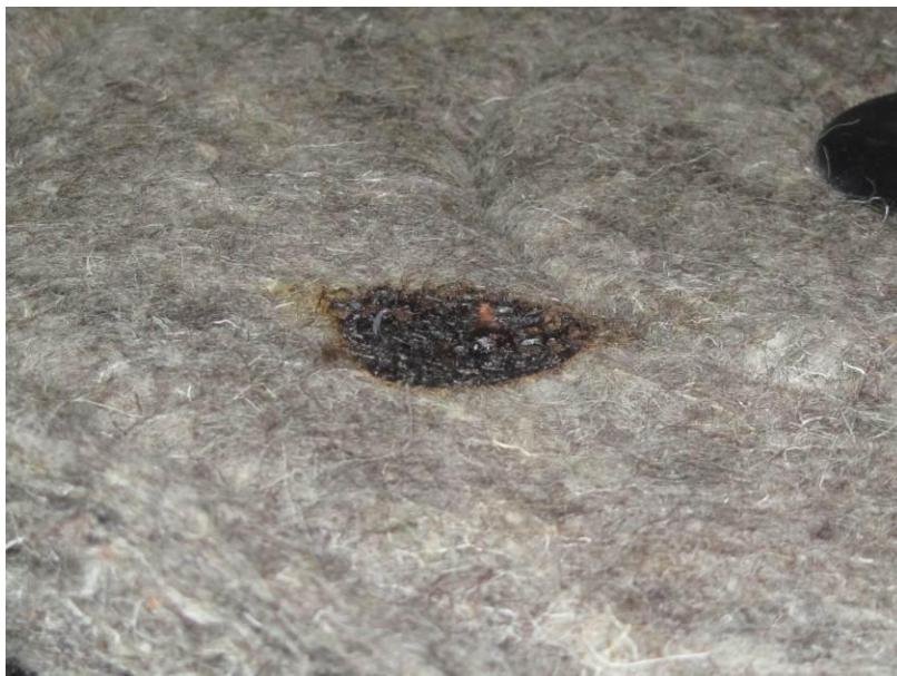
Resultant burn marks after ignition source# 2 test
