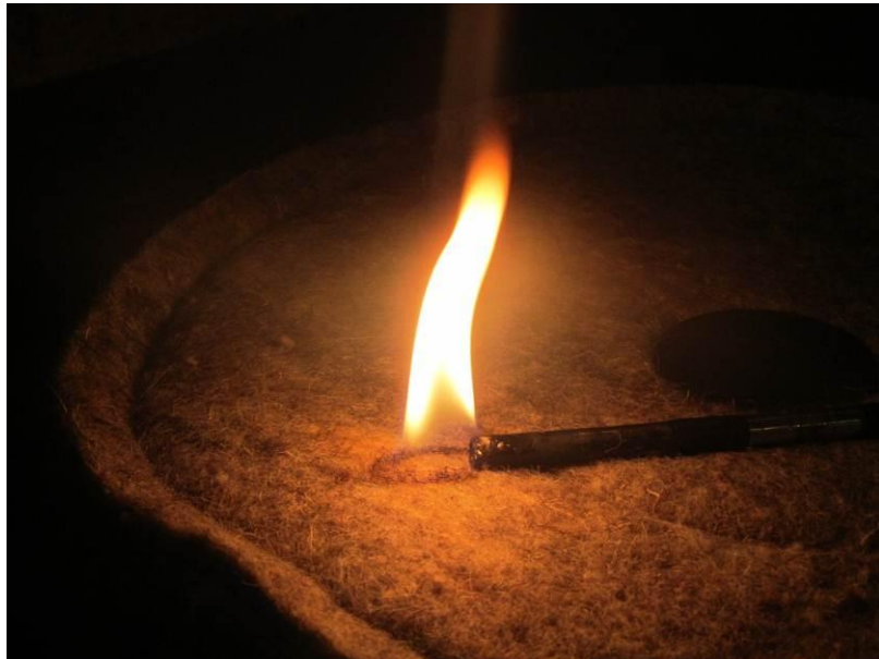
Application of ignition source #2 to upper surface
