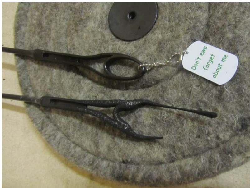
Showing undamaged handle and hang tag and damaged handle after test
