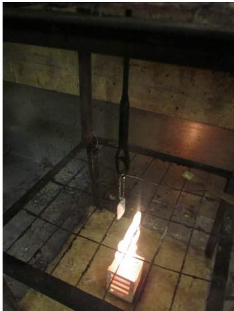
Showing crib 7 test with handle and hang tag in position
