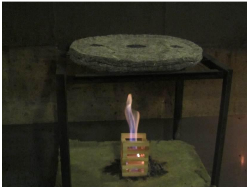
Showing crib 7 ignition source below chimney sheep
