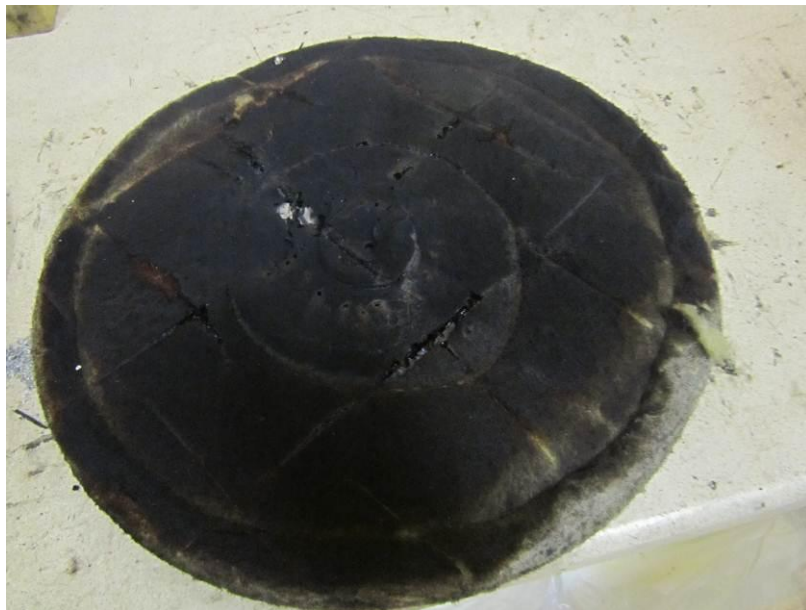
Showing burned underside of chimney sheep after crib 7 test
