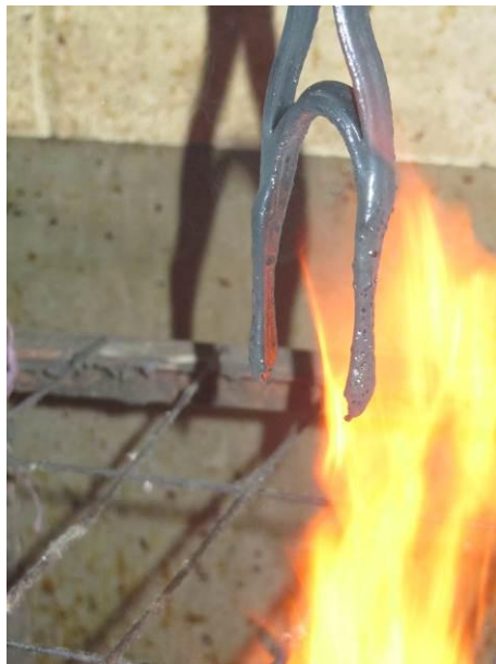
Showing melting plastic handle
