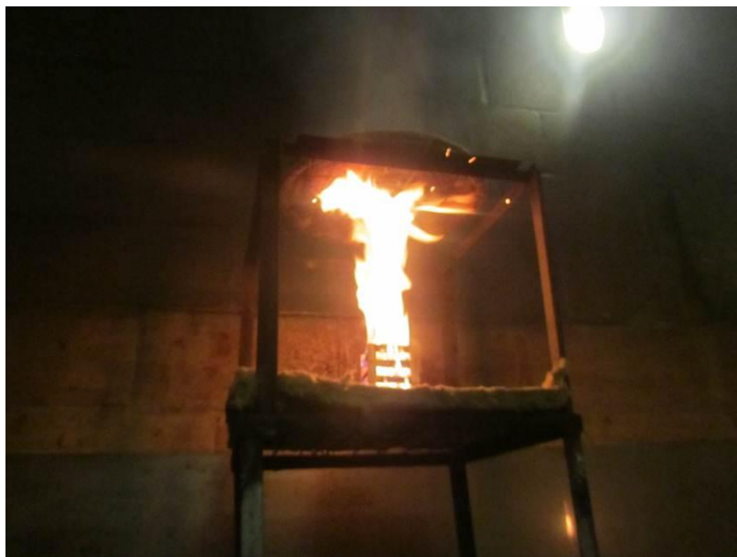
Showing crib 7 ignition source flames on underside of chimney sheep (without handle present)
